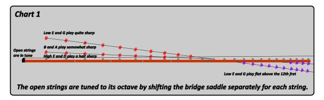
Chart 1 demonstrates that if all open strings are tuned to the octave by shifting the bridge saddle, the fingerboard positions are all out of tune.
