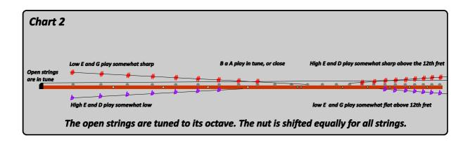
The chart above shows improvement in intonation but points out issues that remain unresolved after the nut is moved forward, as the graph illustrates. Even though this intonation method reduces the maximum disharmony between open strings and notes played on the fingerboard, the intonation error between notes played on the fingerboard remains.
