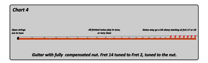
As Chart 4 shows, the tones on the finger board are perfectly in tune even when open strings are tuned. Only the tones played behind the 17<sup>th</sup> fret may sound slightly higher. But let's call a spade a spade, when juxtaposed with the standard method, as presented in Chart 1, this result is beyond compare. Here is a brief explanation of approaching the method of a fully compensated nut:
